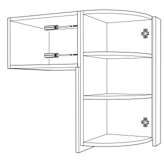
Fix curved wall back panel to rail ' ${f B}$ ', (to right of hinge plate ensures a secure fit).
