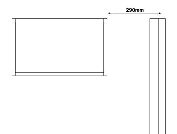
Fix rail 'A' to wall ensuring top of rail aligns with top of adjacent cabinet. **NOTE:** Wall fixing screws have not been provided with this
